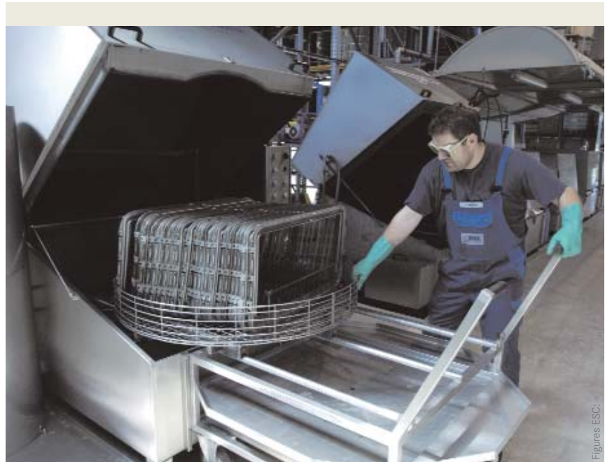
The stripped parts are unloaded by truck.
