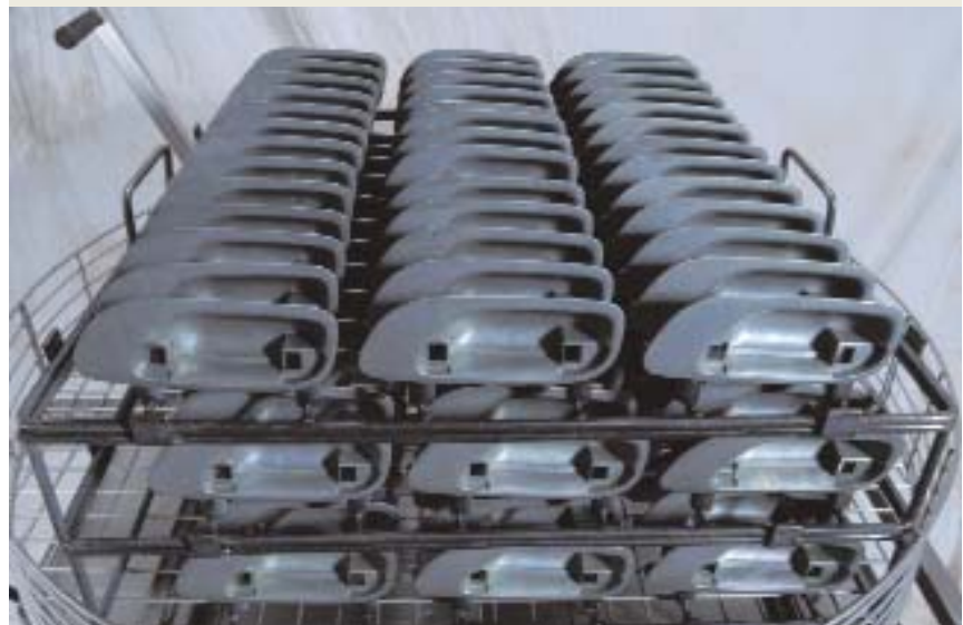
The example of these handles shows how the baskets in the stripping system can be loaded with several layers of parts.
